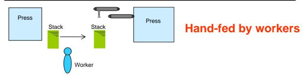
[Countermeasure] Installed a sub-transfer between the presses.
